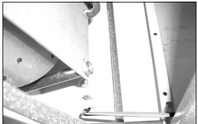
Fig. 49: Release the earthing cable between the cover and the chassis (1)
