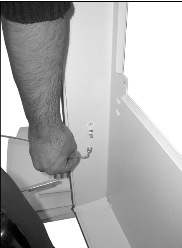
Fig. 73: Disconnect the earthing cable (2)
