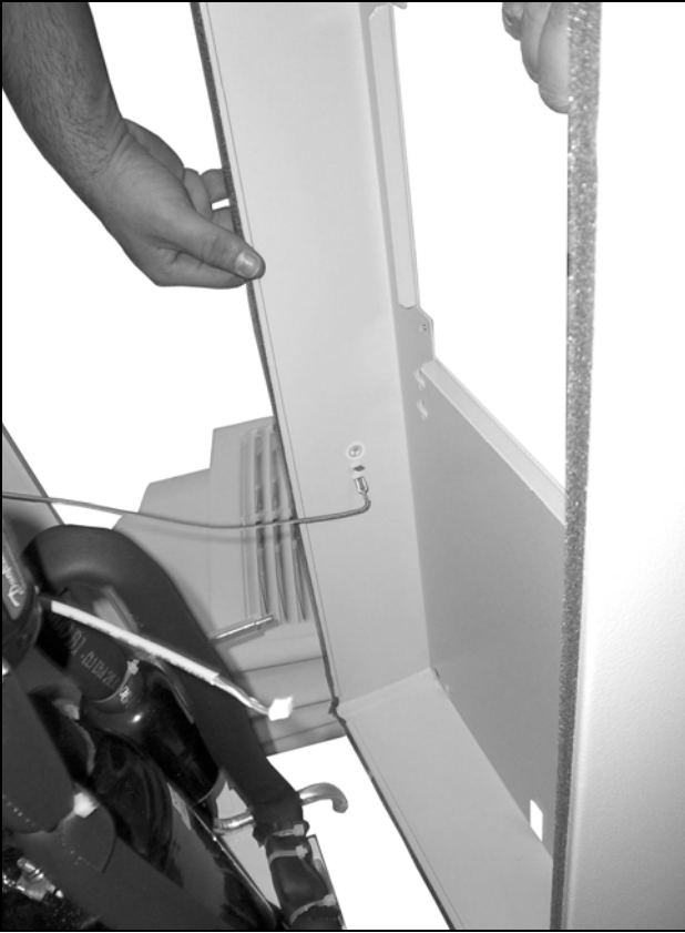
Fig. 72: Disconnect the earthing cable (1)
