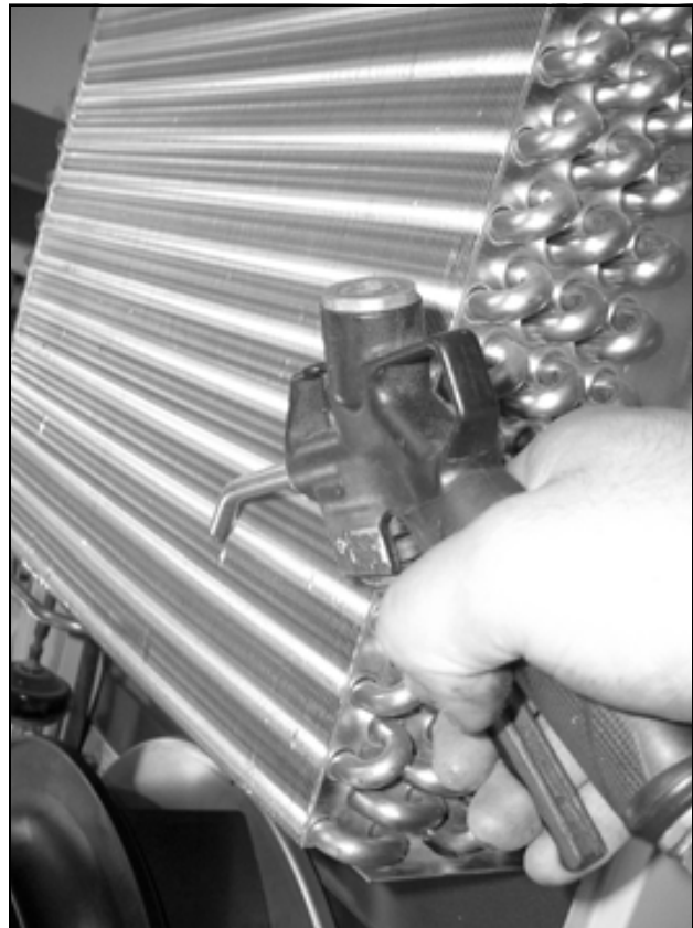
Fig. 75: Clean the heat exchanger coil and compressor chamber using compressed air (2)
