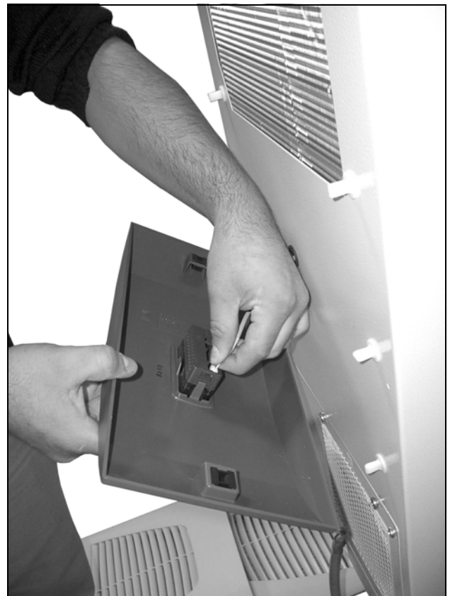
Fig. 38: Disconnect the connector from the display (1)
