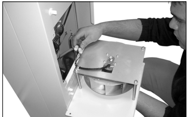
Fig. 65: Disconnect the fan connectors (1)
