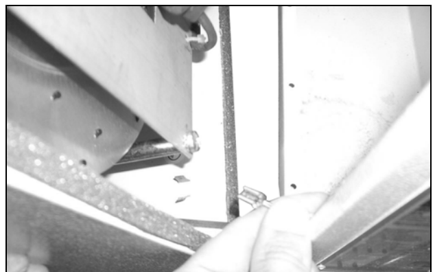
Fig. 50: Release the earthing cable between the cover and the chassis (2)
