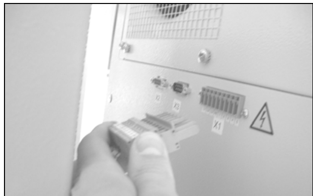
Fig. 34: Disconnect the mains plug
