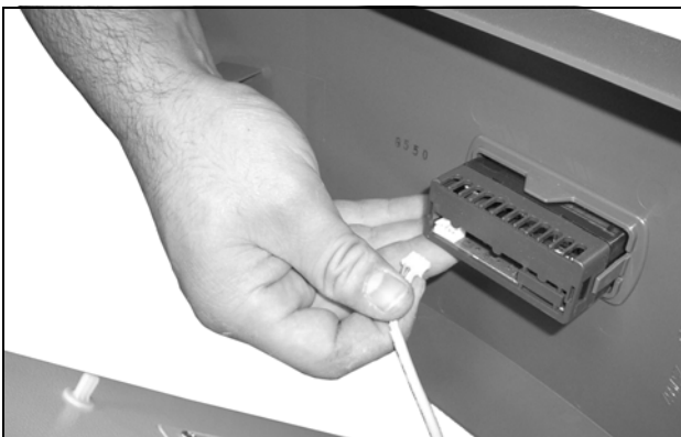
Fig. 60: Disconnect the display cable
