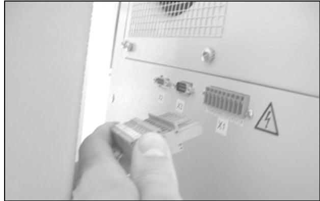
Fig. 53: Disconnect the mains plug
