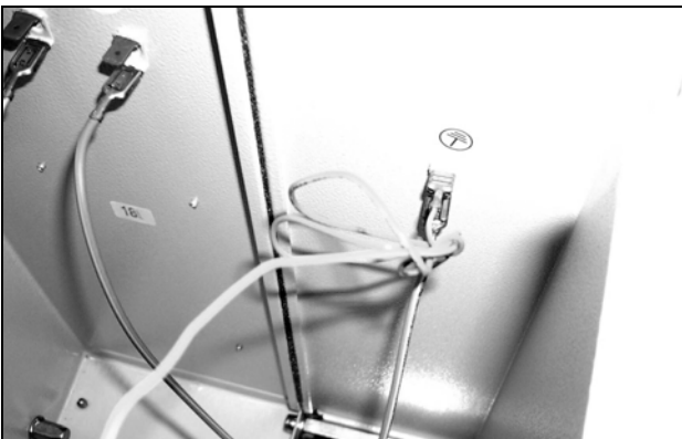
Fig. 68: Disconnect the fan earthing cable (1)
