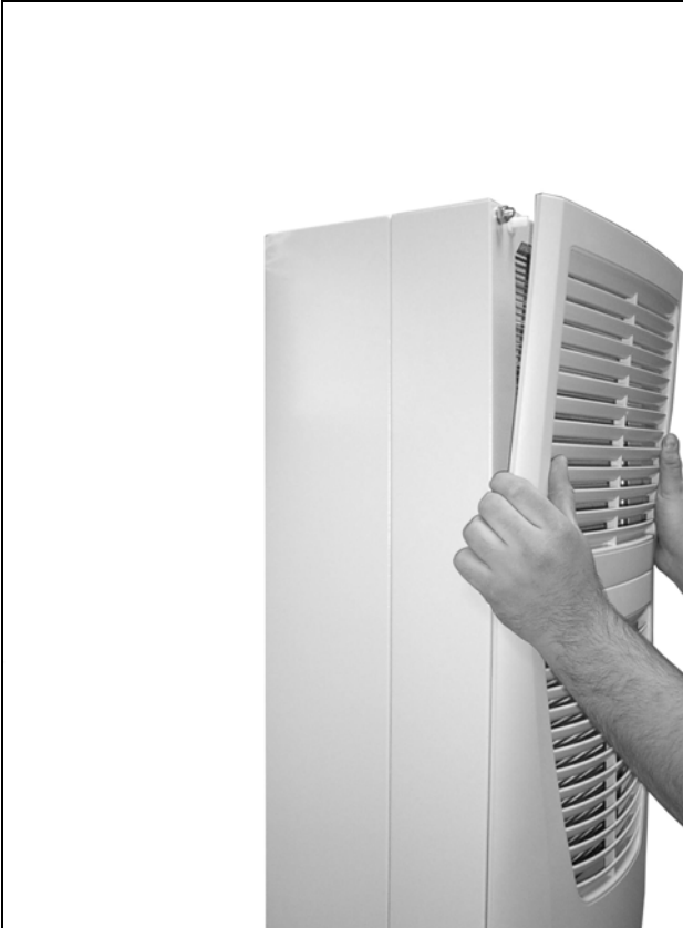
Fig. 55: Remove the top louvred grille (2)
