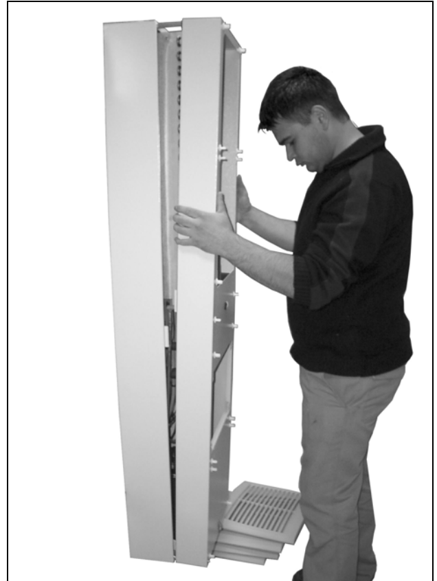
Fig. 71: Removing the cover
