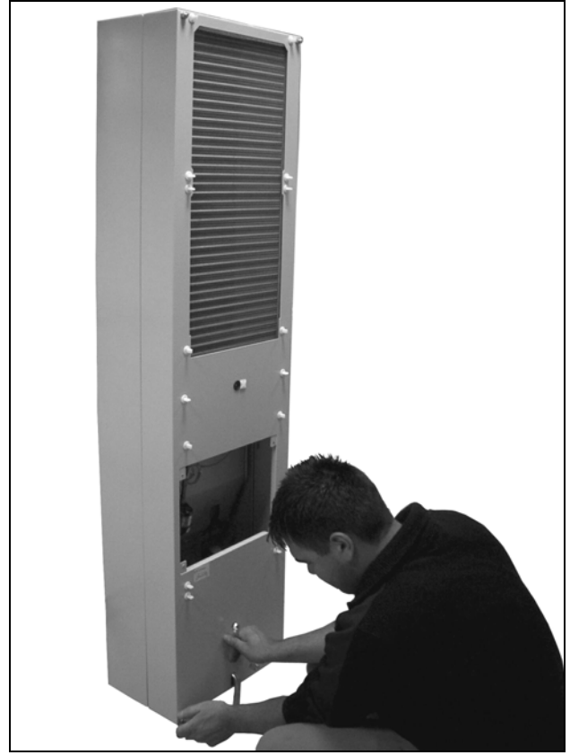
Fig. 70: Undo the four screws for the cover
